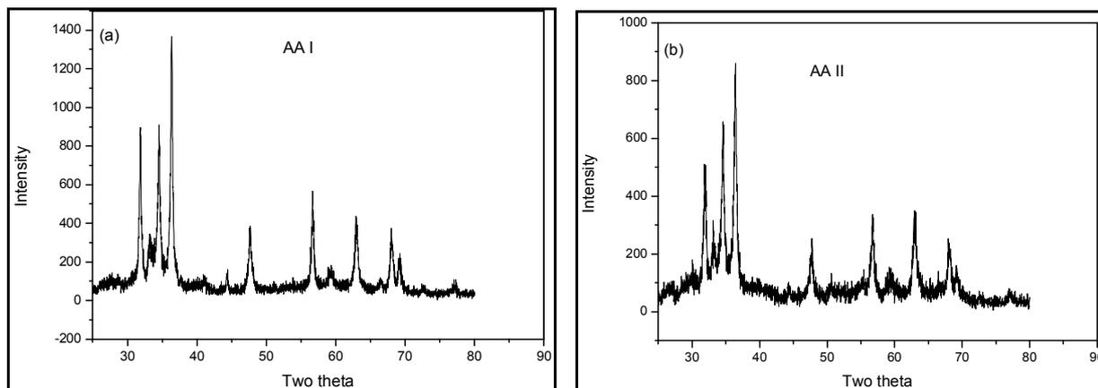
**Fig1: XRD pattern of nano ZnO obtained from  $Zn(CH_3COO)_2$  by Conventional MW irradiation**
