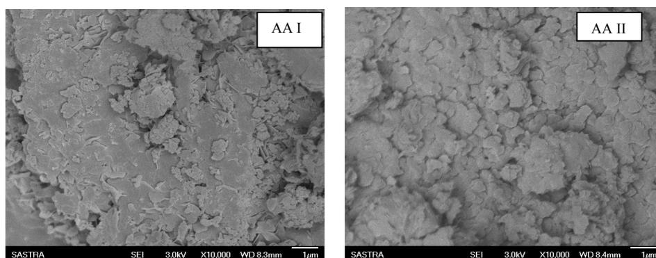
**Fig2. SEM photographs of nano ZnO obtained from  $Zn(CH_3COO)_2$  a) Hot air oven b) MW irradiation**
